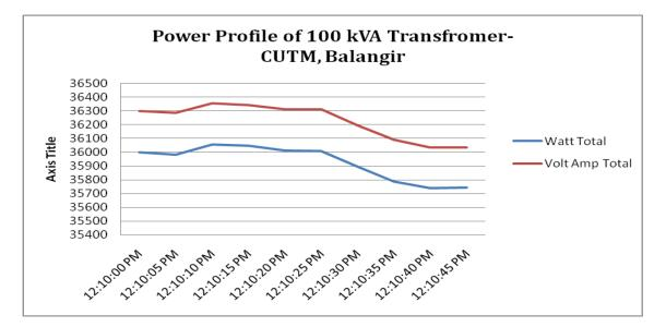
Figure 7: Trend of Load & VA of 100 kVA Transformer-CUTM
