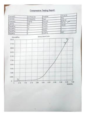
Figure 11 Compressive strength of paving block
