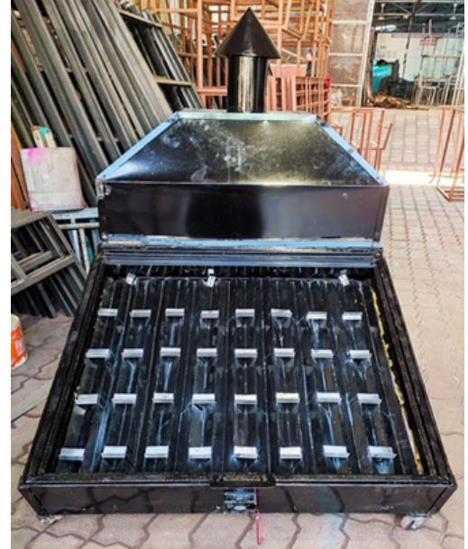
Hybrid Type Solar Dryer with phase change material for drying food products
