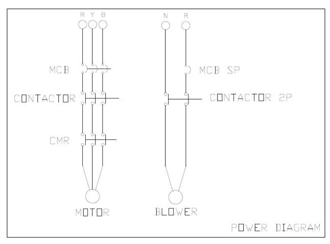
Figure 12: KC DRG ITA Power Diagram
