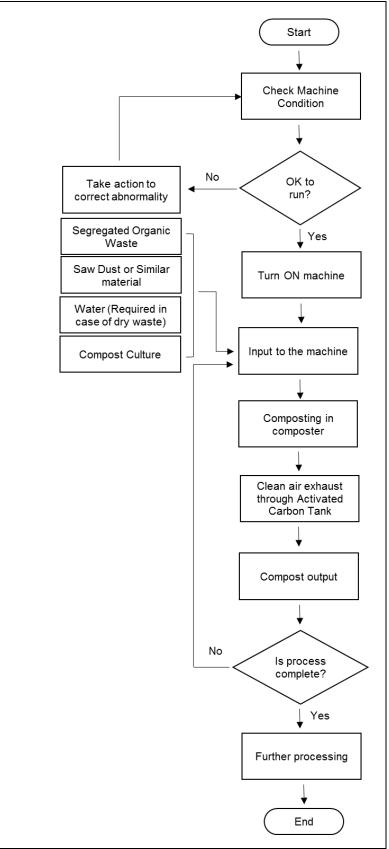
Figure 8: Composting Process Flow Diagram
