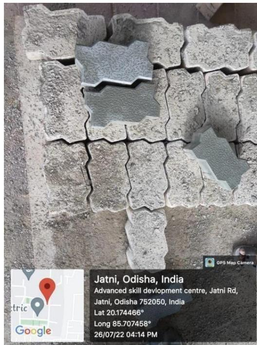
Figure 10 Paving block after removing from mould
