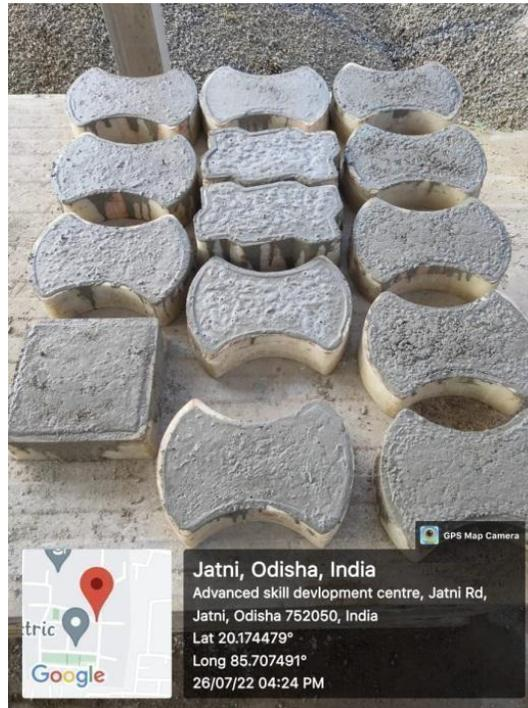
Figure 9 Paving blocks after 24 hours
