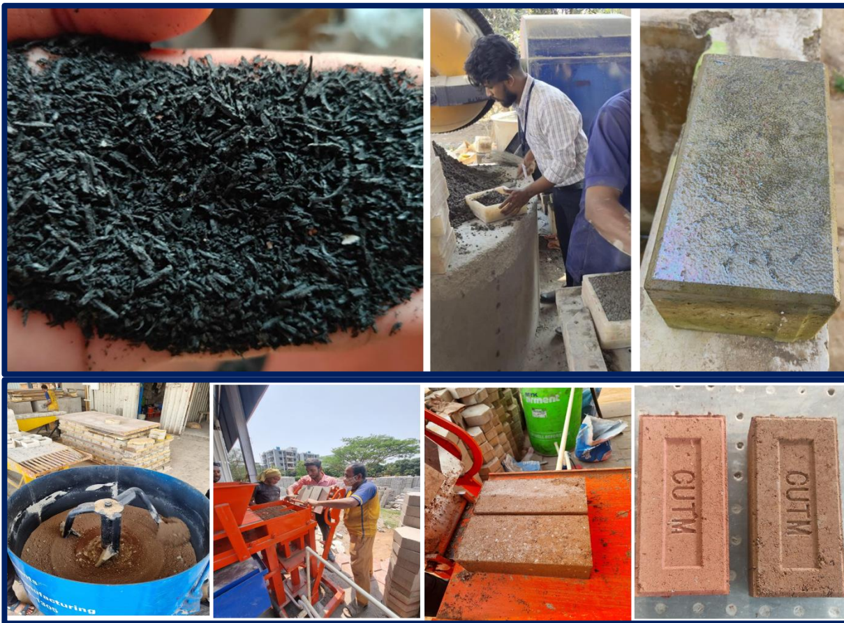
Fig. 22 Paver blocks from scrapped rubber
