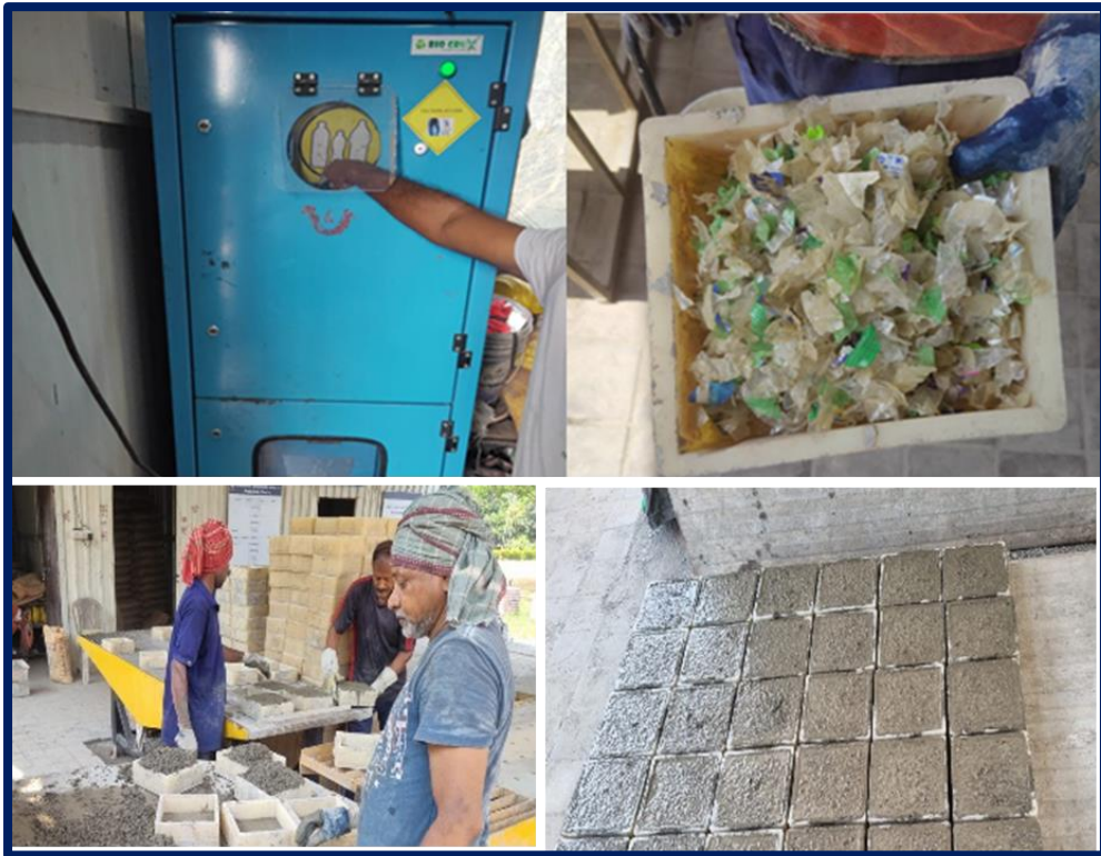
Fig. 18 Paver blocks from waste plastic
