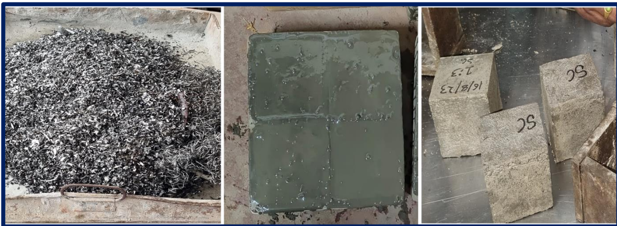
Fig. 21 Paver blocks from scrapped iron
