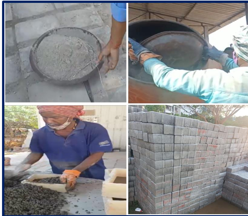
Fig. 20 Paver blocks from Flyash bricks
